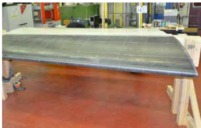
Fig. 6 - Droop Nose mechanical prototype HW
