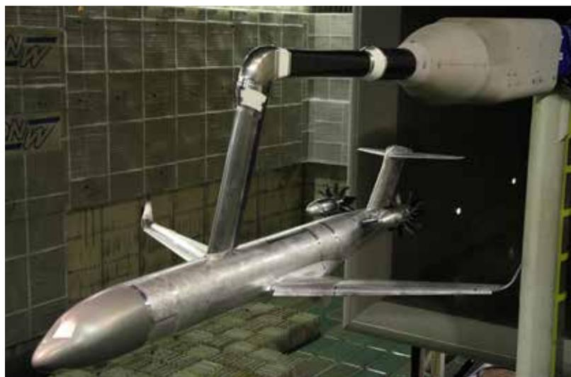
1/7th scale aero-acoustic wind tunnel test model of a CROR powered single aisle airliner with the Airbus CROR blade geometry in the DNW wind tunnel in early 2013. This configuration has also been used for numerical tool development and validation in Clean Sky.
