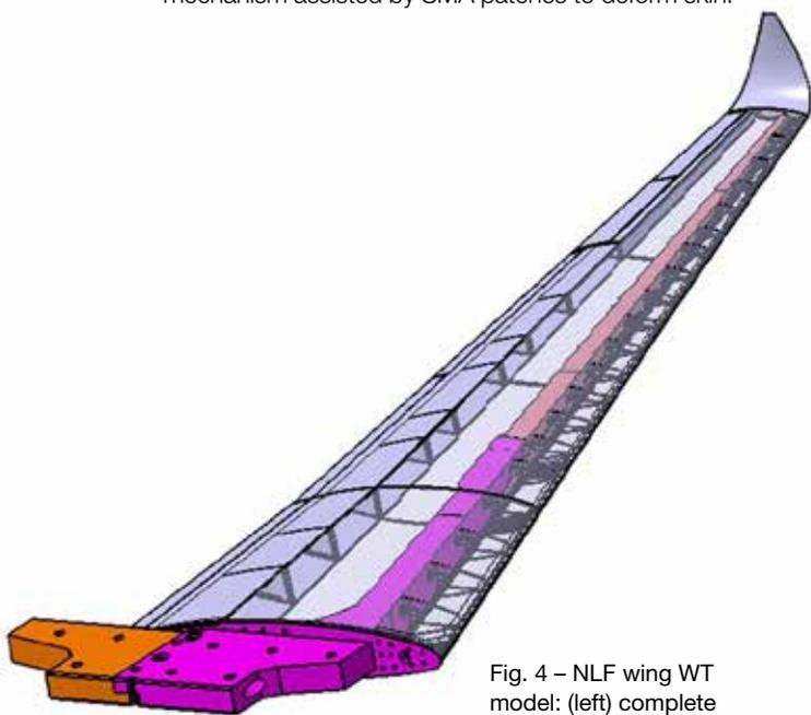
Fig. 4 – NLF wing WT model: (left) complete model CAD geometry; (right) steel outboard spar HW
