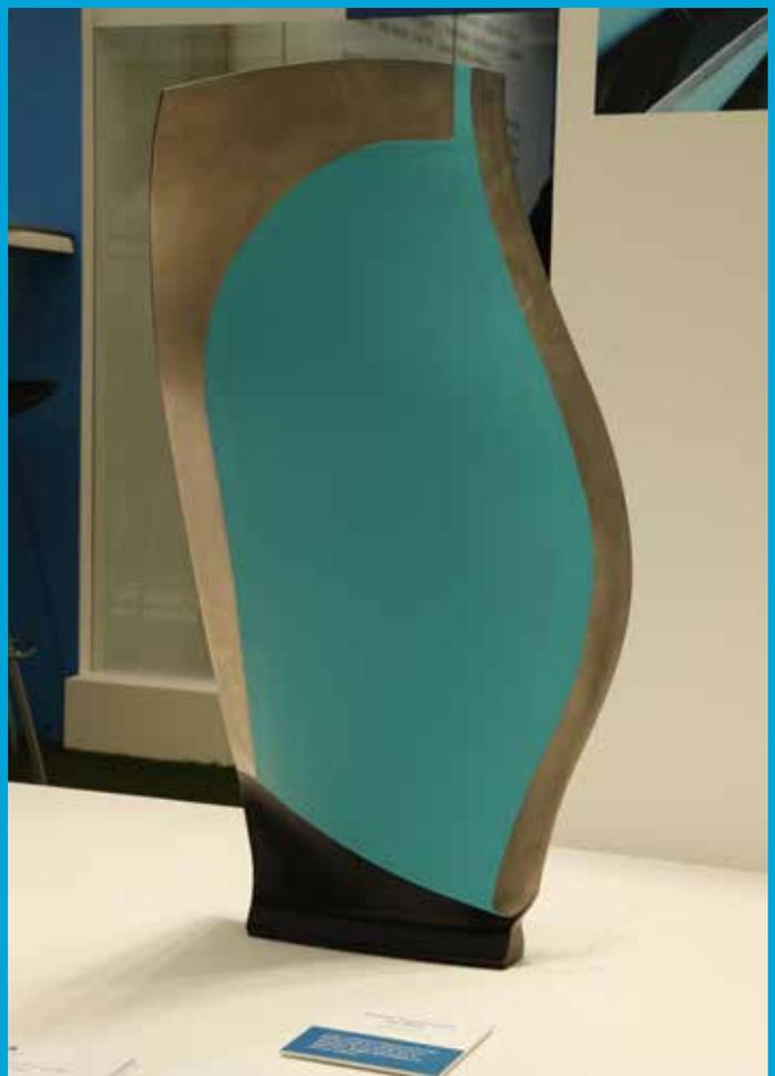
Carbon Titanium (CTi) Fan Blade part of SAGE ITD
