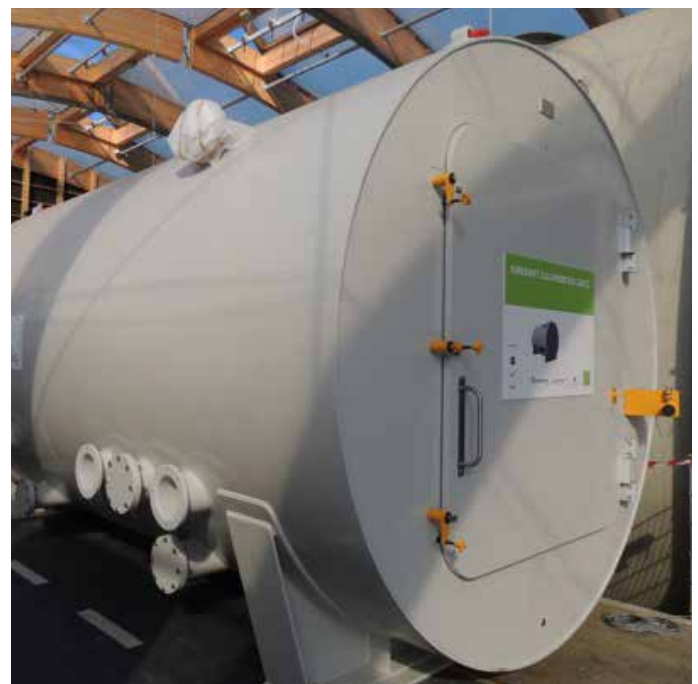
ACC – Aircraft Calorimeter, insulated low pressure steel vessel, internal minimum absolute pressure 0 mbar, internal temperatures -65°C to +120°C
