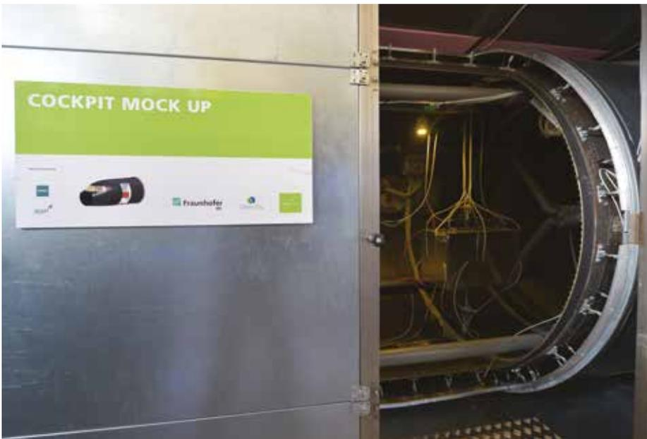
The carbon cockpit mock-up is ready for further measurements.
