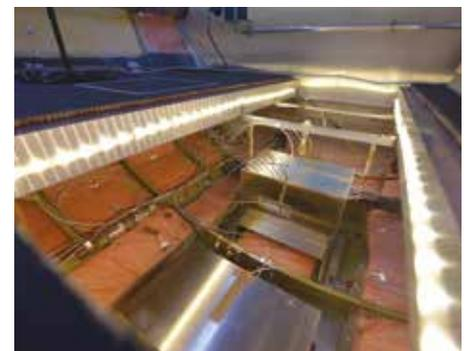
Equipment simulators underneath the floor of the cabin.
