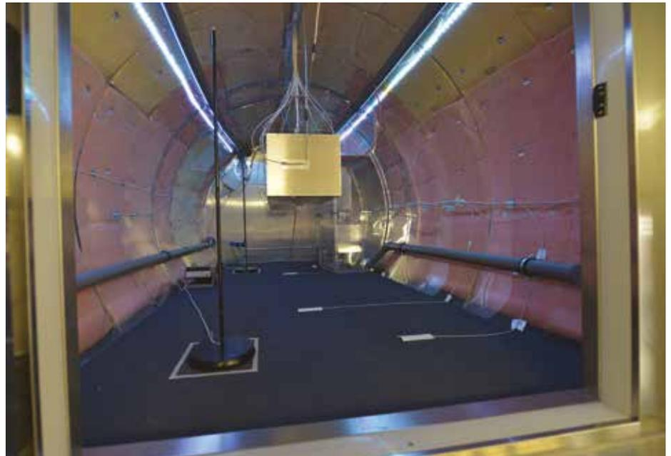
The cabin mock-up is equipped with measuring devices, equipment simulators, original equipment, a fuselage tank section. Integration of realistic cabin interiors is foreseen.
