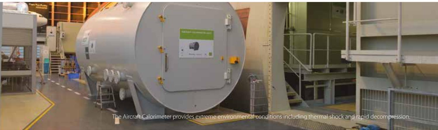
The Aircraft Calorimeter provides extreme environmental conditions including thermal shock and rapid decompression.
